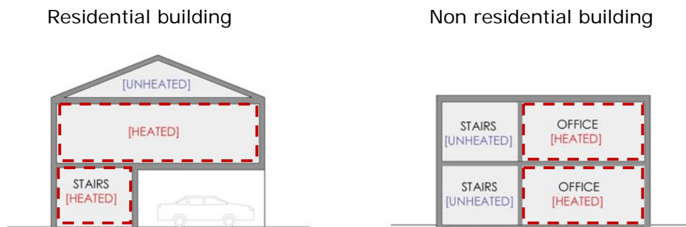
Figure 6: Example section for heated/cooled net volume [internal]
