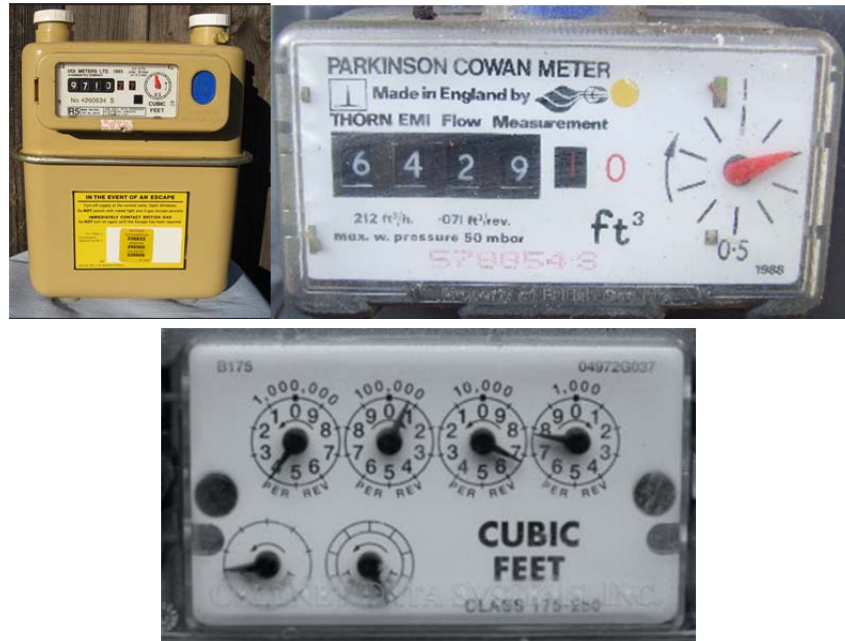
Figure 25. Old analogue gas meter in ft 3 units
